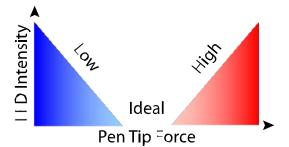
Figure 3: Pen tip force indicating mode where two LED's communicate the ideal force. Different colors and intensity indicate direction and amount of force applied.
